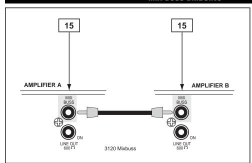
Fig. 20B - Rear Panel Mix Buss Bridging Diagram
